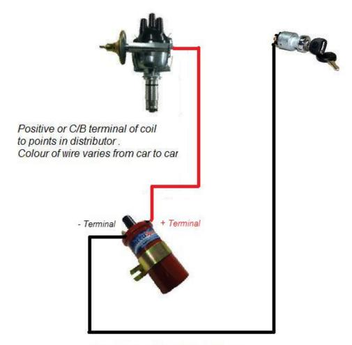
Negative feed from ignition key to negative / SW side of coil colour of wire varies from car to car
